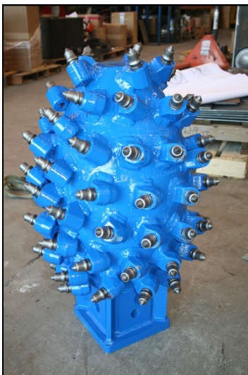
Left: "Football" profiler head with carbide tips Right: Conical profiler head with carbide tips
