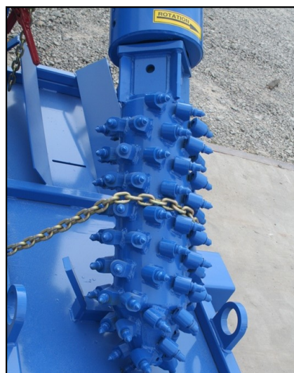
Left: "Football" profiler head with carbide tips Right: Conical profiler head with carbide tips
