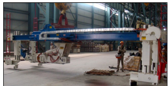
GEF-530-72R with optional cable management system
