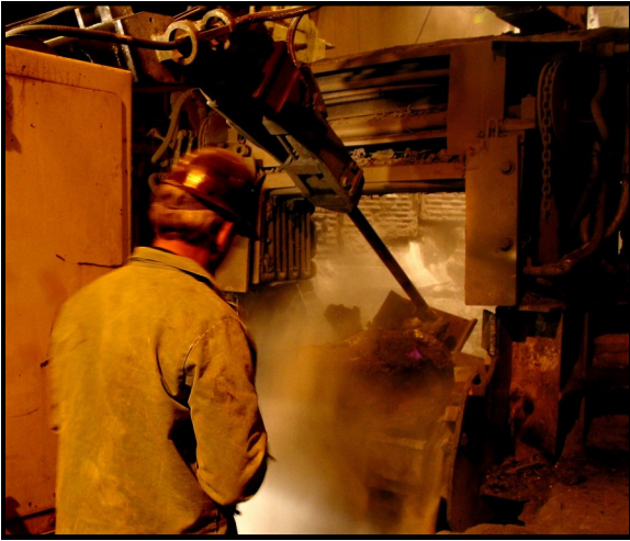
SCRAPING DEBRIS FROM EAF FURNACE
